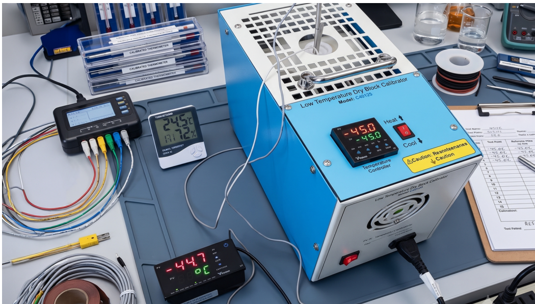
Dry block calibrator used for industrial temperature probe calibration
