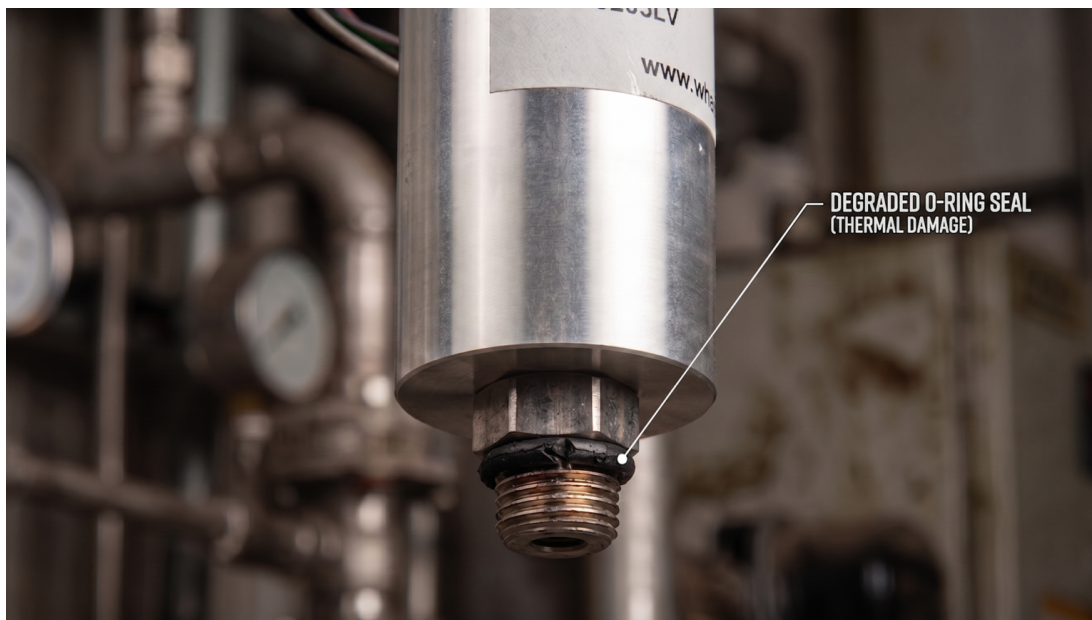
Close-up of O-ring seal on a vacuum switch wetted component showing signs of thermal degradation in an industrial setting
