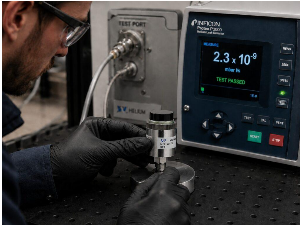
Technician performing helium leak testing on a sealed sensor unit.
