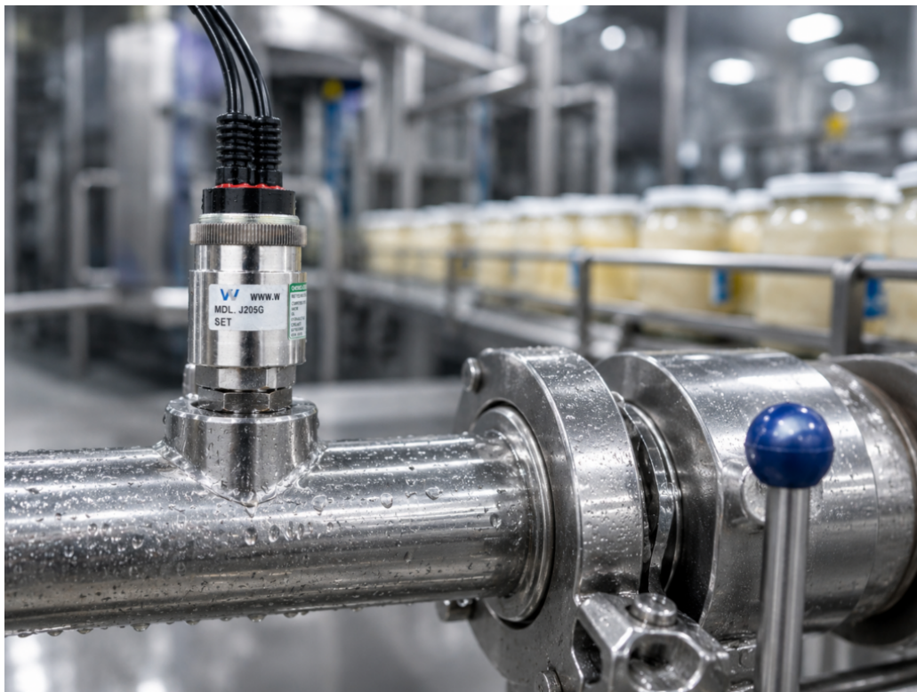
Sanitary stainless steel pressure switch in food processing line
